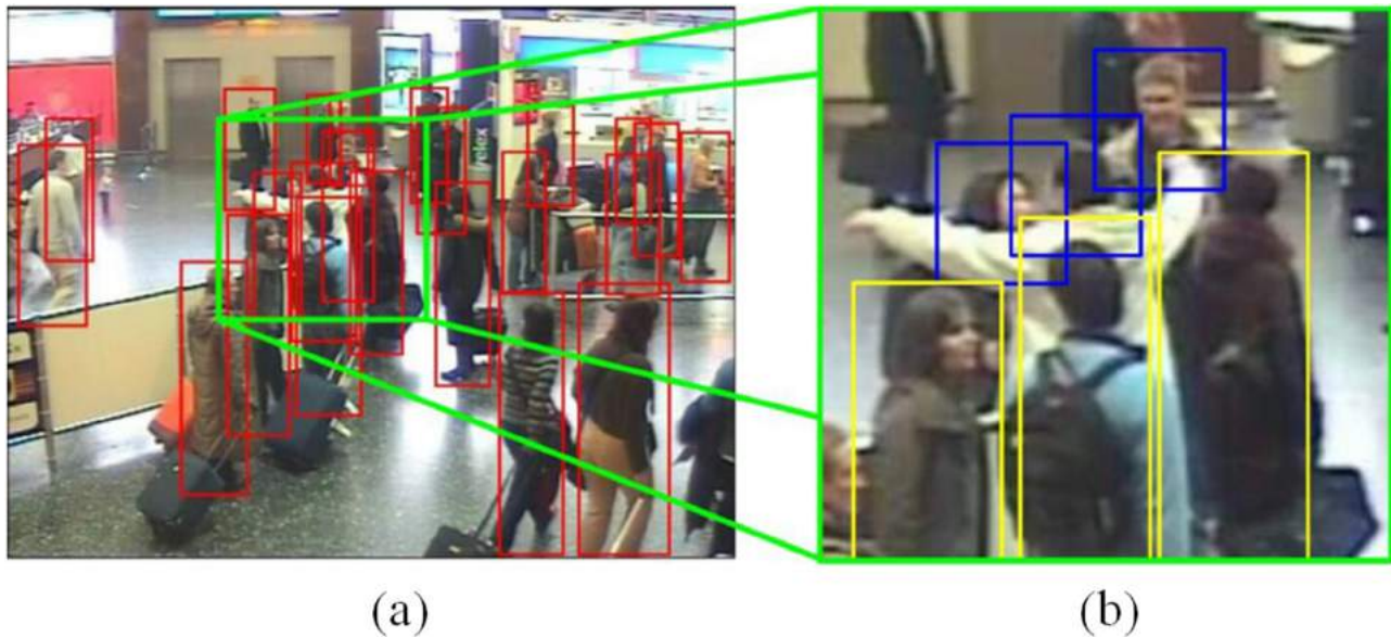
Fig. 3. (a) An annotation example from SED-PD. Red bounding boxes denote the pedestrians. (b) Partial details. Pedestrians in blue boxes are heavily occluded by pedestrians in yellow boxes. (For interpretation of the references to color in this figure legend, the reader is referred to the web version of this article.)
